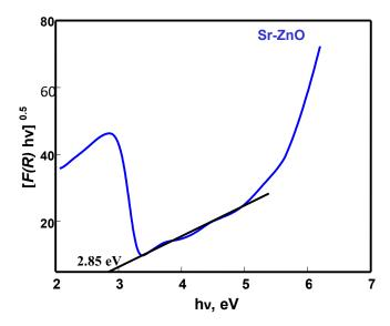
Fig.5 Tauc plot for Indirect Band Gap Energy of Sr-ZnO
