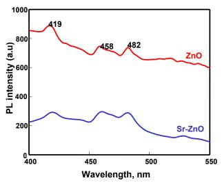
Fig.6 Photoluminescence Spectra of Sr-ZnO and ZnO
