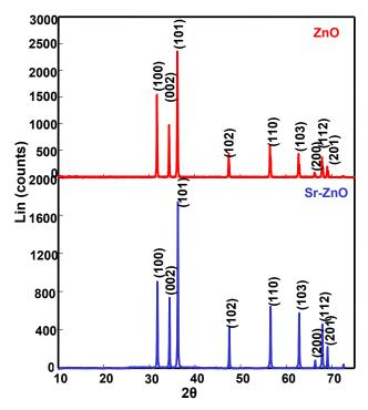
Fig.1 Powder X-ray Diffraction Spectra of Sr-ZnO and ZnO
