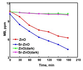
Fig.7 Temporal Profiles of Degradation of Methylene Blue Dye under Visible Light
