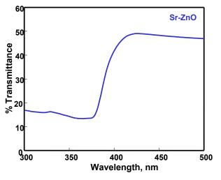
Fig.4 Transmittance Spectrum of Sr-ZnO
